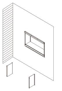
7. Insert the front glass panel back in place after the media installation has been completed.
