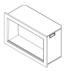
5. Put the fireplace into the wall opening and fix it to the wall by screwing 2 screws each side.
